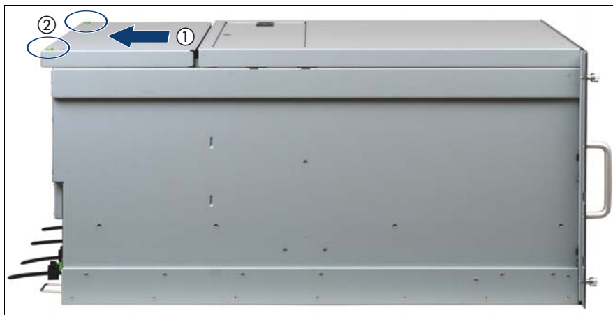
Figure 7: Removing the rear cover
